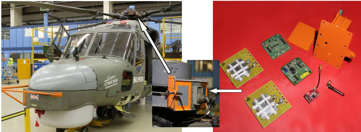
*Fig. 8: WISD hardware and installation on the helicopter.*
